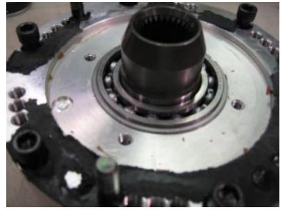
3. REMOVE THE FOUR SOCKET HEAD BOLTS SECURING INPUT SEAL RETAINER FROM PLANETARY HOUSING AND REMOVE SEAL RETAINER.
