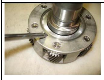
6. REMOVE SNAP-RING FROM THE PLANETARY AS-SEMBLE. THIS SNAP RING SECURES THE INPUT SHAFT INTO SIX GEAR PLANETARY ASSEMBLY.
