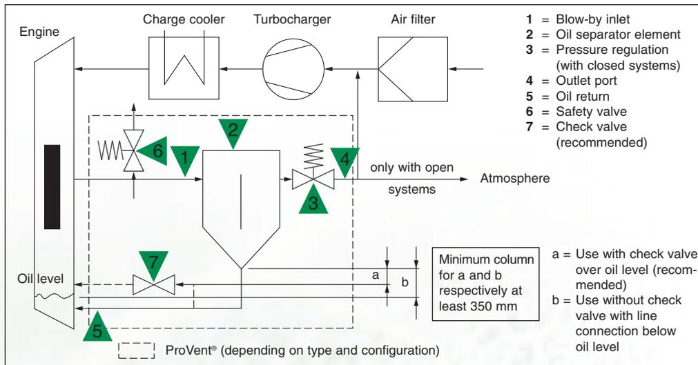
Fig. 2: Diagram of closed and open crankcase ventilation
