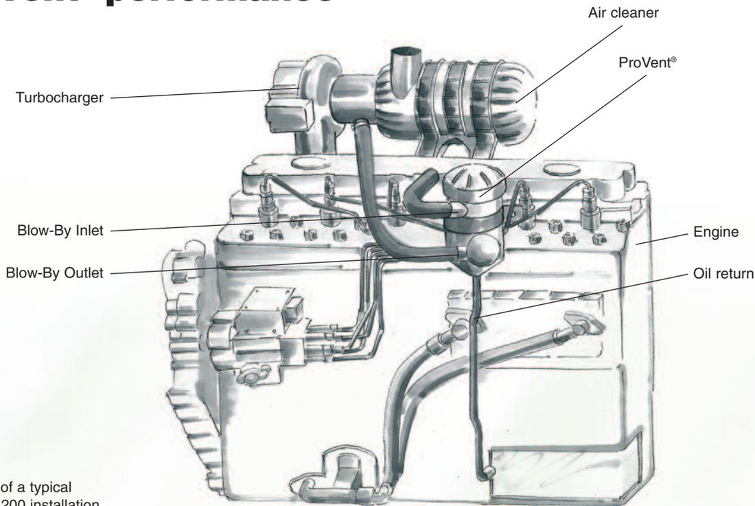
Example of a typical ProVent® 200 installation.
