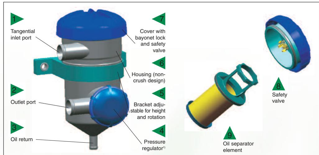
Fig. 1: Components with example of ProVent® 200 <sup>1)</sup> only effective with closed systems
