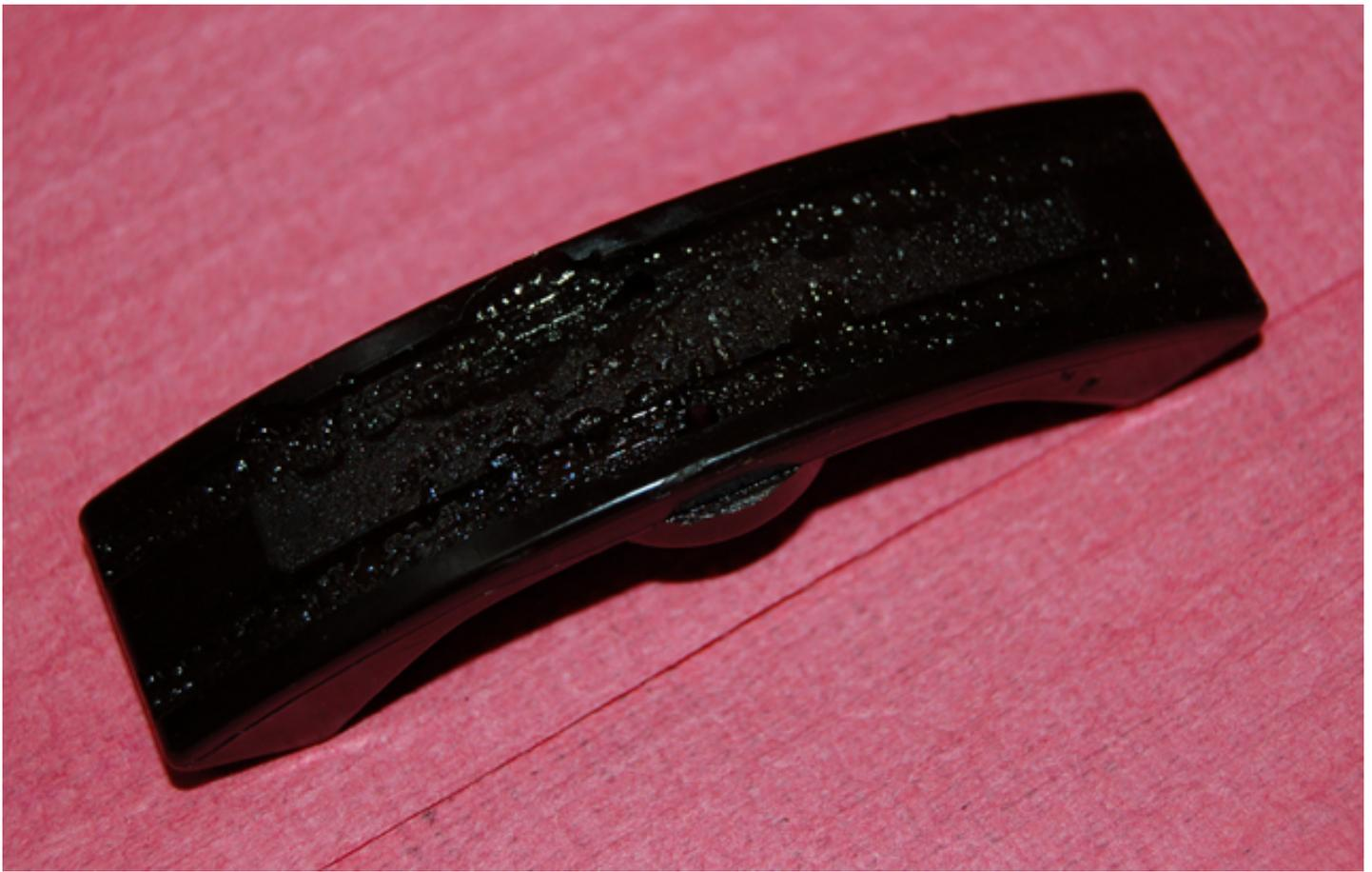
cam chain tensioner pad, 2.5 Boxster M96 engine, using Mobil 1 0w40 at factory recommended drain intervals, ~75,000 mi.
