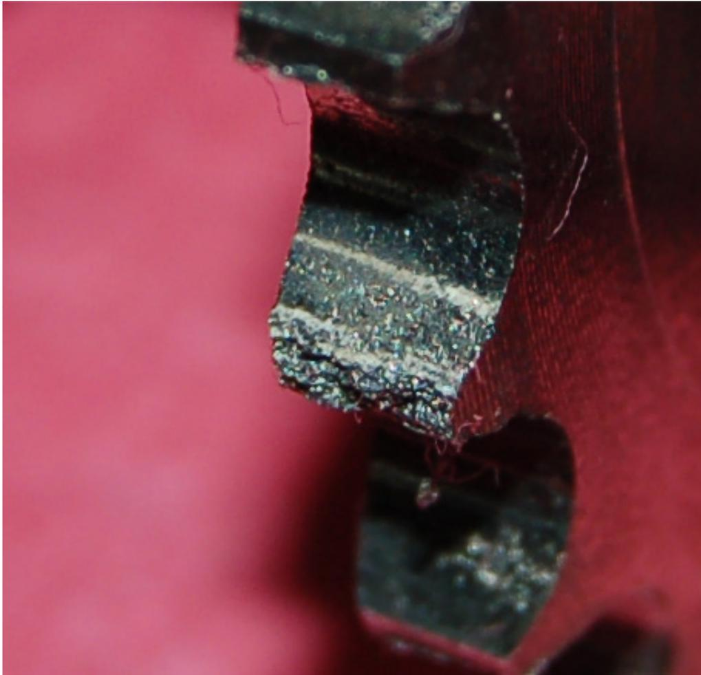
cam sprocket wear, 2.5 Boxster M96 engine, using Mobil 1 0w40 at factory recommended drain intervals, ~35,000 mi.
