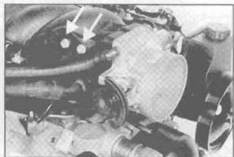
Install 1/4-20 thread inserts in manifold to mount throttle linkage bracket (if required).
