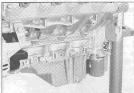
The LS1 block has multiple bosses that can be used for custom engine mounts.
