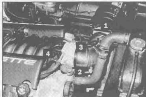
1. PN 25179711 Air meter 2. PN 12160244 Intake Air Temperature (IAT) sensor 3. PN 25147210 Duct (curved) - includes IAT sensor 4. Plug EGR port.
