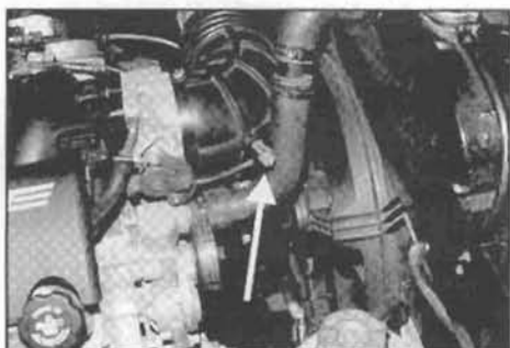
Intake Air Temperature (IAT) sensor PN 12160244
