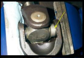
17. Stop when the snapring groove is inside the yoke
