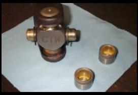
14. Continue by removing the cpas from the remaining 2 trunnions, and installing an o-ring followed by snapring onto both.
