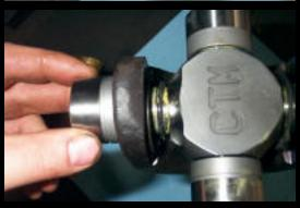
5. Carefully install a bearing cap on the trunnion by pressing it through the hole in the axle yoke.
