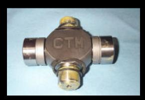
1. Take a joint, remove a pair of opposing bearing caps, and onto each trunnion place a snapring followed by an o-ring.
