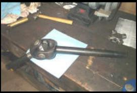
22. Before installing the axle assemblies into the axle housing - do a final check that all yokes move smoothly and freely with no binding; that all caps are greased and grease fittings are installed; and that all snaprings are firmly seated in the groove and do not spin under finger pressure.
