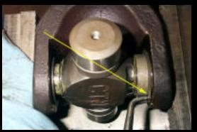
9. Install snapring in snapring groove using snapring pliers (yellow arrow)
