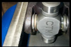
12. Remember to pause and slip the snapring over the cap, press cap until snapring groove is visible inside yoke, and insert snapring in groove
