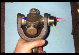
10. Place the other cap on its trunnion (yellow arrow) and using the brass or hardwood drift tap the joint in the direction indicted by the red arrows to seat the snapring (blue arrow) tightly between the flat on the inside of the yoke and the snapring groove in the cap. Set the cap and snapring in this manner so that you cannot spin the snapring in its groove with finger pressure.
