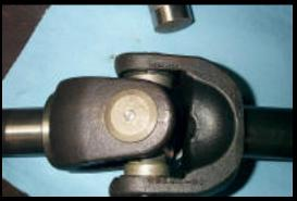
21. Install the grease fittings in the ends of each of the caps and grease the U-joint at each cap with a high quality synthetic grease..
