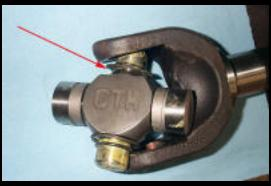
2. Hold the cross so the CTM label faces you and the cut-out is at the top facing you. Place the snapring in the cut out area (red arrow) and slip this trunnion into the yoke first.
