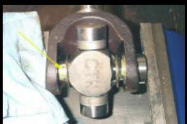
6. Once the cap is lined up and finger tight proceed to press it in using your vice or shop press. When doing the first one, be sure to use a rag to protect the end of the opposite trunnion (yellow arrow) from being marred by the jaws of the vice.
