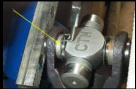
7. Pause partway once the cap protrudes past the inside flat of the yoke. Spread the snapring with pliers and slip it over the cap (yellow arrow).
