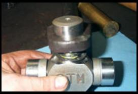
Start by using your fingers, being extra careful to keep he trunnions, caps, and yoke bores all lined up, and making sure the o-rings and snaprings aren't pinched or caught up...
