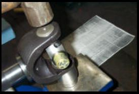
13. You must also press joint back in opposite direction to seat cap and snapring. I found it necessary to place cap over a large socket and tap the opposite cap to seat the snapring
