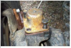
Step one, remove existing kingpin cap (or stock steering arm) bolts / studs. If they've been there for a while, significant force / heat may be required.
