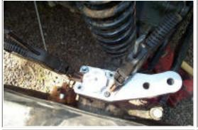
Use a couple of clamps to cinch down the arm on the studs so that you can start the nuts on the studs.
