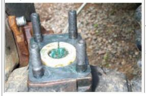
When all the studs are installed, wipe away excess thread locking compound from the knuckle face, grease both sides of a new gasket, and install it over the studs.
