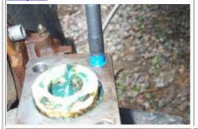
Install the studs in the knuckle, and torque to 80 ft .lbs.
