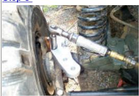
Once the nuts are started, sequentially tighten down the nuts, which will eventually clamp the steering arm down over the studs and in place on the knuckle.
