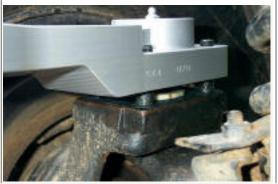
Then place the OTT steering arm over the studs. It will not drop all the way on, because of the kingpin spring, and also because of the tight tolerances between stud and holes.
