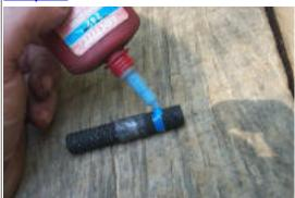
Apply thread locking compound to the SHORT end of the studs.
