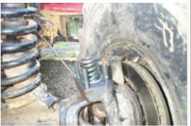
Place the spring retainer and spring back in place on top of the kingpin bushing
