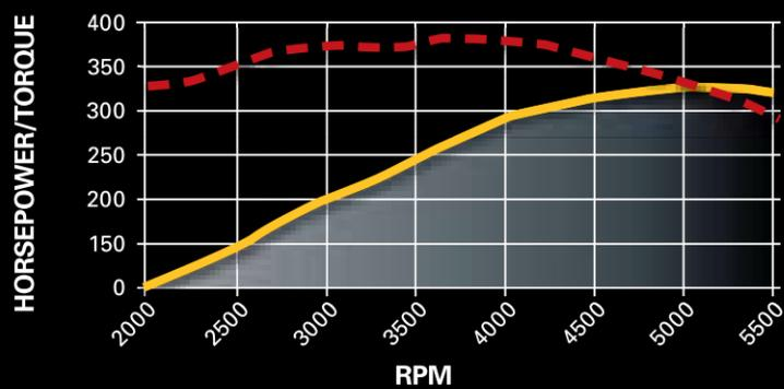
Horsepower: 355 @ 5250 rpm      Torque (lb-ft): 405 @ 3500 rpm
