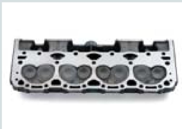
**A** Cast-iron Vortec Cylinder Head (combustion chamber)
