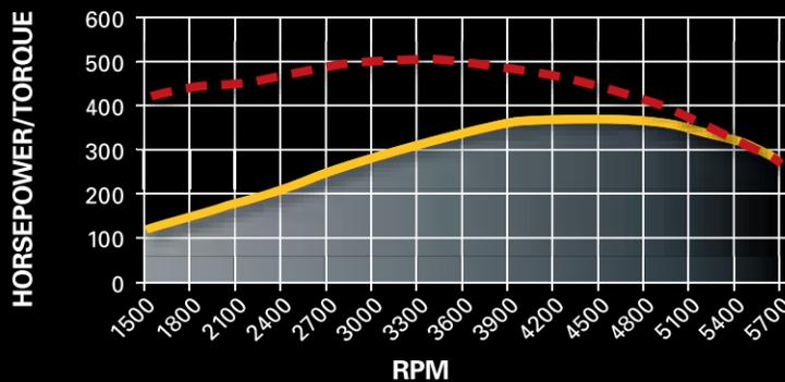
Horsepower: 377 @ 4500 rpm      Torque (lb-ft): 512 @ 3300 rpm
