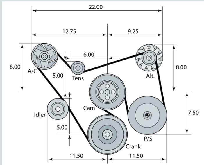
**A** Serpentine Accessory Drive System (with air conditioning): Diagram
