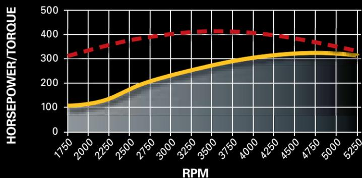
Horsepower: 340 @ 4500 rpm      Torque (lb-ft): 435 @ 4000 rpm
