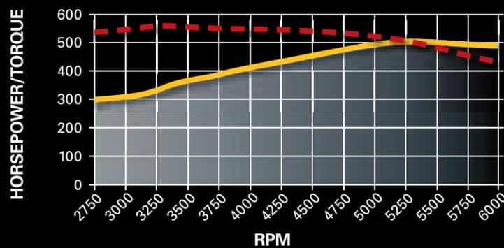
**Horsepower: 502 @ 5100 rpm**      **Torque (lb-ft): 565 @ 3200 rpm**
