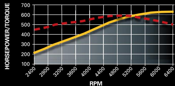
Horsepower: 620 @ 6200 rpm
