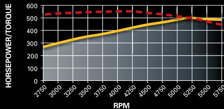
**Horsepower: 502 @ 5200 rpm**      **Torque (lb-ft): 567 @ 4200 rpm**
