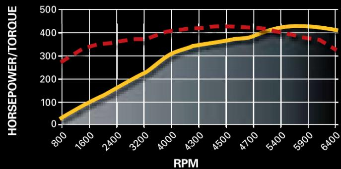
Horsepower: 430 @ 5900 rpm      Torque (lb-ft): 424 @ 4600 rpm
