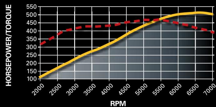
Horsepower: 515 @ 6500 rpm      Torque (lb-ft): 469 @ 5000 rpm
