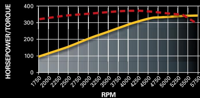
Horsepower: 350 @ 5800 rpm      Torque (lb-ft): 365 @ 4000 rpm
