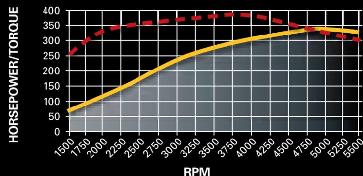
Horsepower: 330 @ 5000 rpm      Torque (lb-ft): 380 @ 3800 rpm
