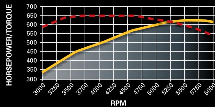
**Horsepower: 620 @ 5500 rpm**      **Torque (lb-ft): 650 @ 4500 rpm**
