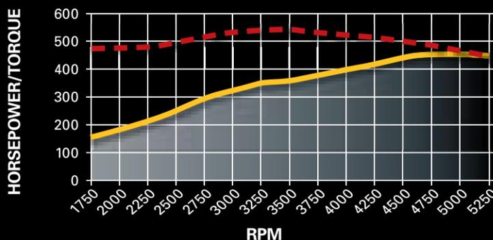
Horsepower: 450 @ 5250 rpm      Torque (lb-ft): 550 @ 3500 rpm
