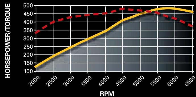
Horsepower: 480 @ 5750 rpm      Torque (lb-ft): 475 @ 4500 rpm
