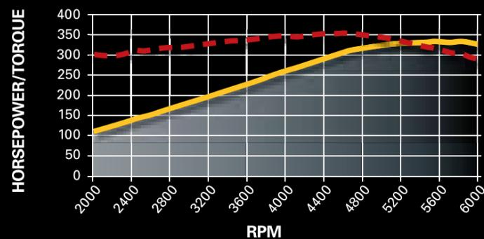
Horsepower: 327 @ 5500 rpm      Torque (lb-ft): 347 @ 4600 rpm
