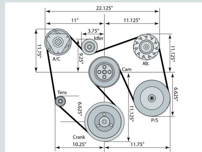
Serpentine Accessory Drive Belt System (with Air Conditioning): Diagram **F**
