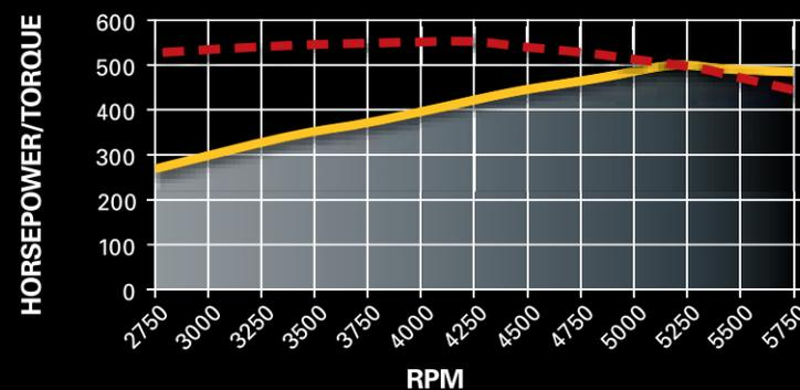
Horsepower: 502 @ 5200 rpm
