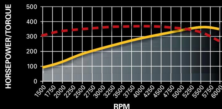
Horsepower: 385 @ 5600 rpm      Torque (lb-ft): 385 @ 4000 rpm
