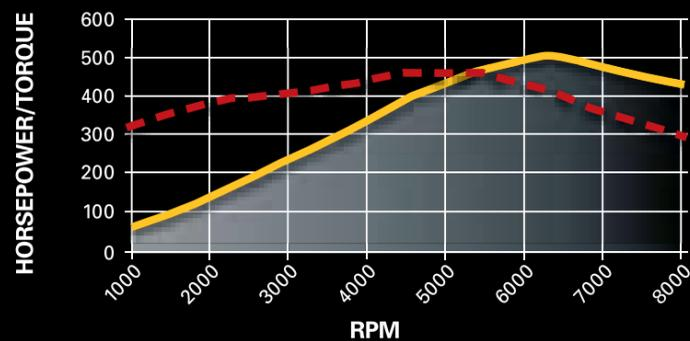
Horsepower: 505 @ 6300 rpm      Torque (lb-ft): 470 @ 4800 rpm
