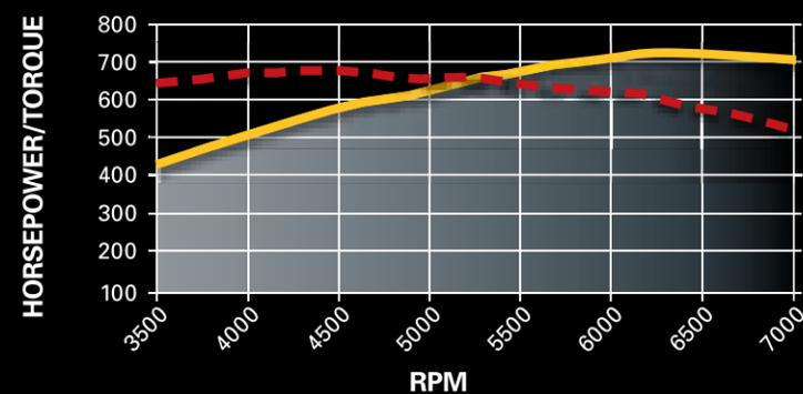
**Horsepower: 720 @ 6250 rpm**      **Torque (lb-ft): 685 @ 4500 rpm**
