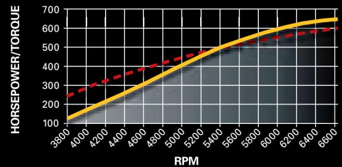
Horsepower: 638 @ 6500 rpm      Torque (lb-ft): 604 @ 3800 rpm
