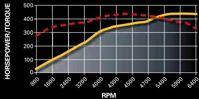
**Horsepower: 450 @ 5900 rpm**      **Torque (lb-ft): 444 @ 4600 rpm**
