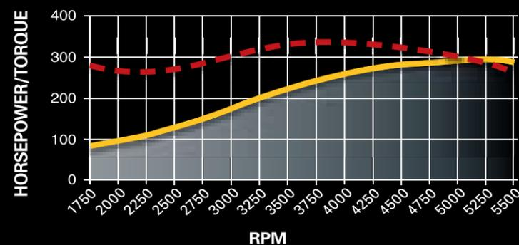
Horsepower: 290 @ 5250 rpm      Torque (lb-ft): 332 @ 3750 rpm
