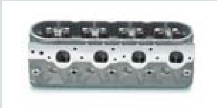
**B** LS7 Cylinder Head Assembly (exhaust)
