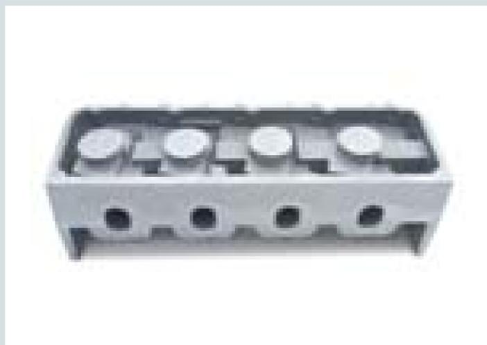
**A** DRCE 2 Raw Aluminum Cylinder Head (intake)
