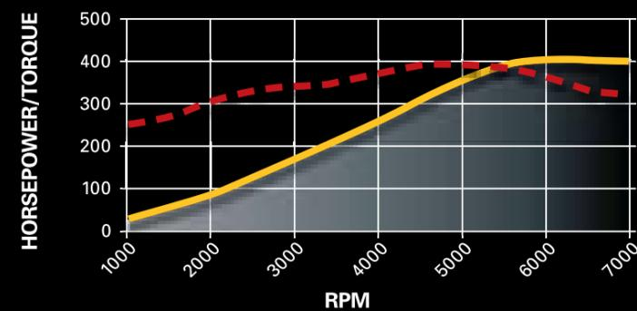
Horsepower: 405 @ 6000 rpm      Torque (lb-ft): 395 @ 4800 rpm
