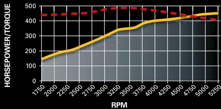
Horsepower: 425 @ 5250 rpm      Torque (lb-ft): 500 @ 3250 rpm
