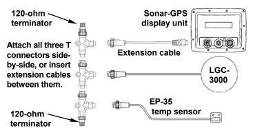
Lowrance NMEA 2000 network with display unit, GPS module and temp sensor.
