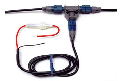
OEM factory installations typically use a Power Node similar to this to supply power to the network bus. The red and black leads are connected to a switched power source, allowing the user to turn off power to the bus.
