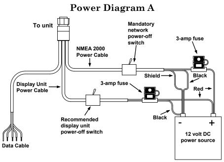
Use this method if you are powering the display unit and a GPS module or the display unit and a NMEA 2000 network.
