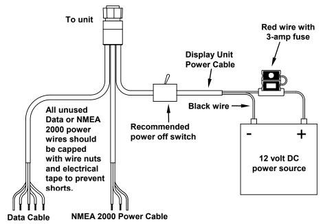
Use this method if you are *only* powering your display unit and are not powering a NMEA 2000 network or any NMEA 2000 accessory device, including a GPS module.
