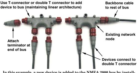
In this example, a new device is added to the NMEA 2000 bus by installing a T connector between a T connector and a terminator at the end of the backbone (network bus).
