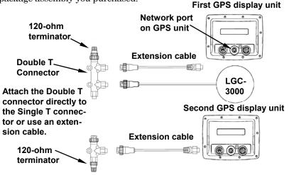
**NMEA 2000 network with LGC-3000 connected to two GPS display units.** The diagram below shows how to expand the network by adding an EP-35 Temperature Sensor. The sonar-GPS display unit would receive the GPS signal from the LGC-3000 and temperature information from the temp sensor.
