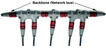
This network bus has a cluster of single and double T connectors and is terminated on both ends. It is connected to a display unit and four NMEA 2000 devices.
