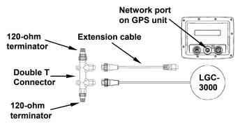
LGC-3000 and GPS display unit as an expandable NMEA 2000 network.
