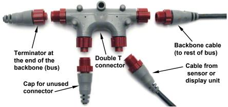
NMEA 2000 network node located at the end of a NMEA 2000 backbone. NOTE:
