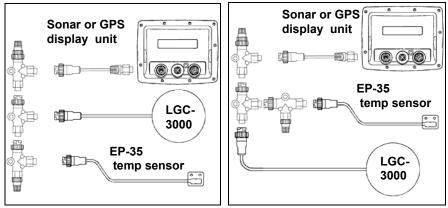
Two possible network designs. The design on the left maintains a linear architecture while the one on the right does not. You should always maintain linear architecture when building a NMEA 2000 network.
