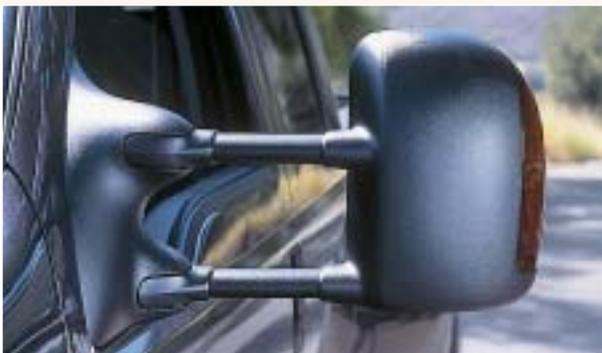
**Extendible mirrors** require less space than conventional towing mirrors when retracted, and offer a clear view of the trailer when they're in position while towing.
